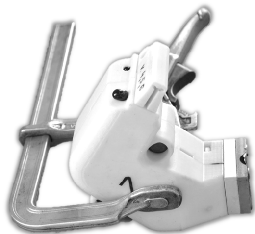
Figure 7. Mold after injection of PUR foam.
