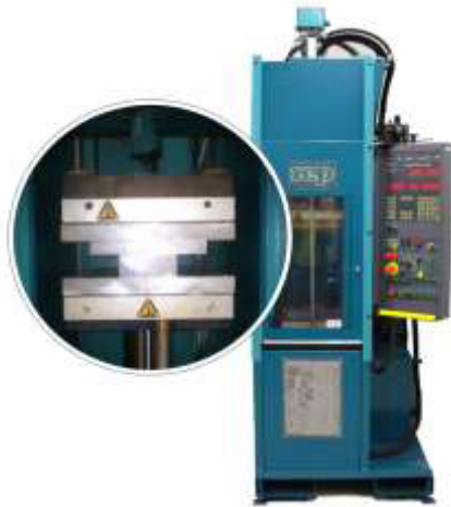
Figure 4. Injection molding machine REP V27/Y125 with injection mold
