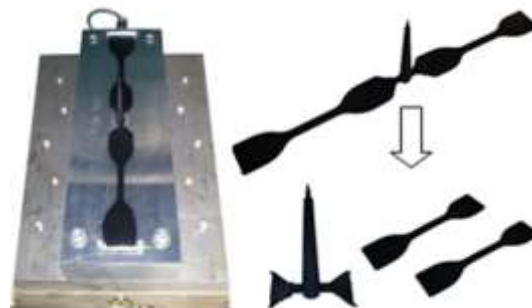
Figure 3. Production of testing samples by injection molding
