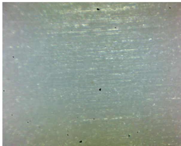
Figure 6. 100 times magnified surface of TPE irradiated by 198 kGy after 15 minutes at 200 °C.
