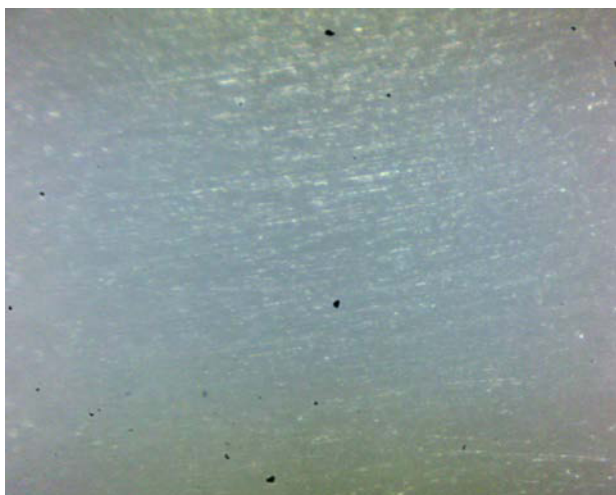
Figure 4. 100 times magnified surface of TPE irradiated by 99 kGy after 15 minutes at 200 °C.
