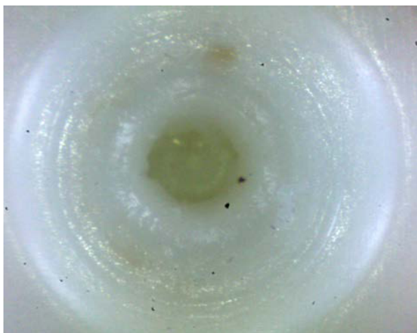
Figure 4. 100 times magnified indentation mark into irradiated PBT by 132 kGy after 5 seconds of penetration at 300 °C.
