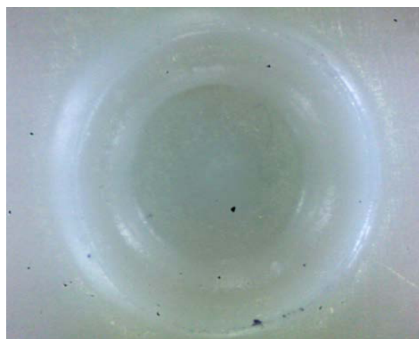
Figure 3. 100 times magnified indentation mark into irradiated PBT by 132 kGy after 5 seconds of penetration at 250 °C.
