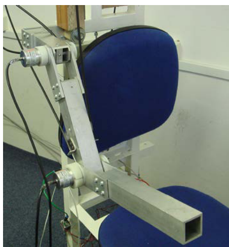
Figure 1. Rehabilitation device driven by pneumatic artificial muscles
