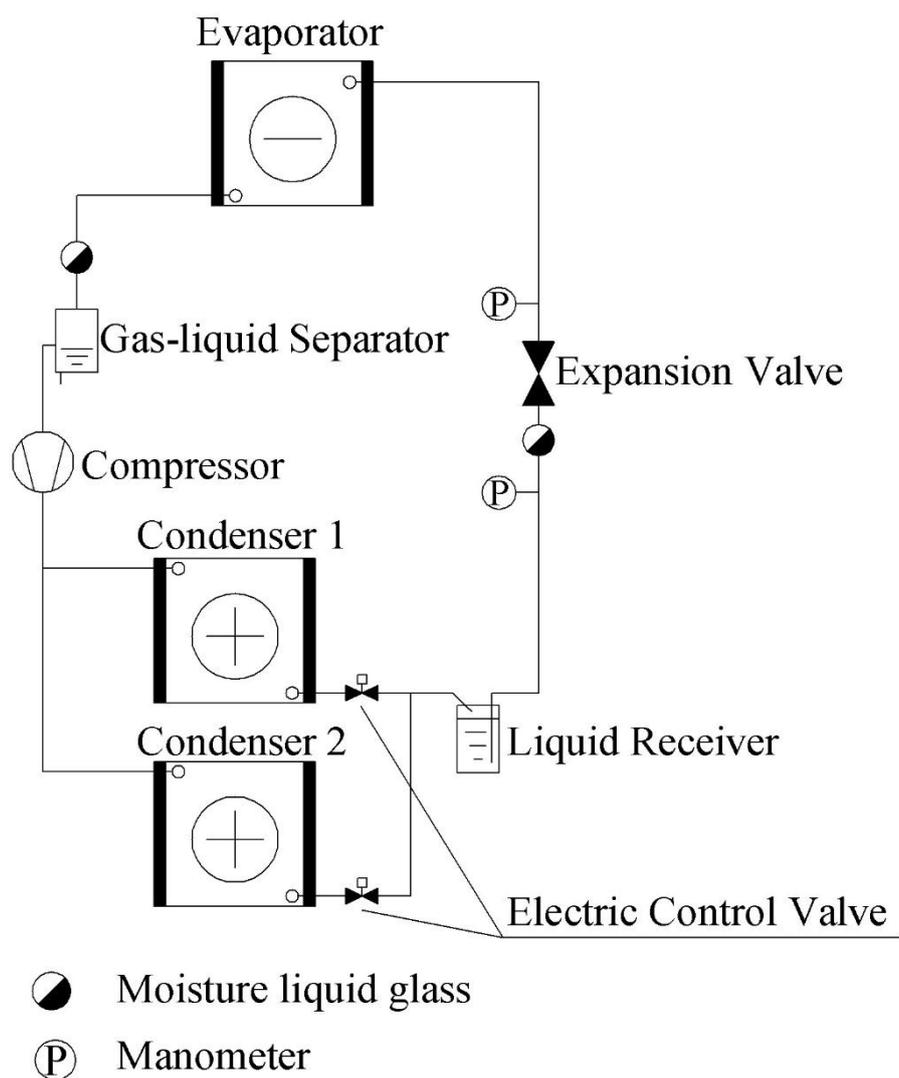
Figure 3. Heat pump designed for the HP-SDC
