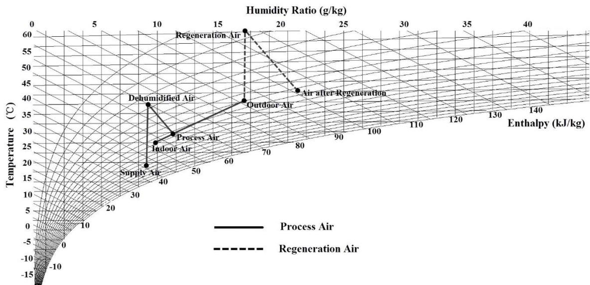
Figure 5. Thermal conditions of ventilation air and regeneration air under Colombo extreme summer class
