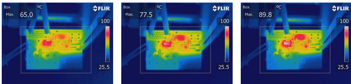
(a) V_{IN} = 37 \text{ V} , F_{SW} = 6 \text{ MHz} (b) V_{IN} = 48 \text{ V} , F_{SW} = 6 \text{ MHz} (c) V_{IN} = 57 \text{ V} , F_{SW} = 6 \text{ MHz}
