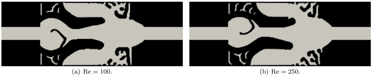
Fig. 4 Example results at different Reynolds numbers.
