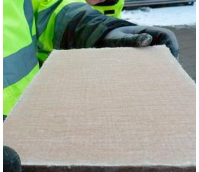
Fig. 1. (a) Sketch of a typical façade construction where a sheathing board is used as wind barrier. Adapted from [1]; (b) Photo of 8 mm thick MgO-board with a glass fibre mesh on both surfaces.
