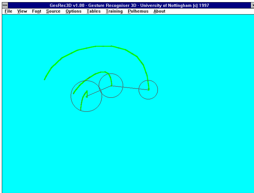
Fig. 2. Traces from 3 sensors attached to the elbow, wrist, and finger (shown left to right)
