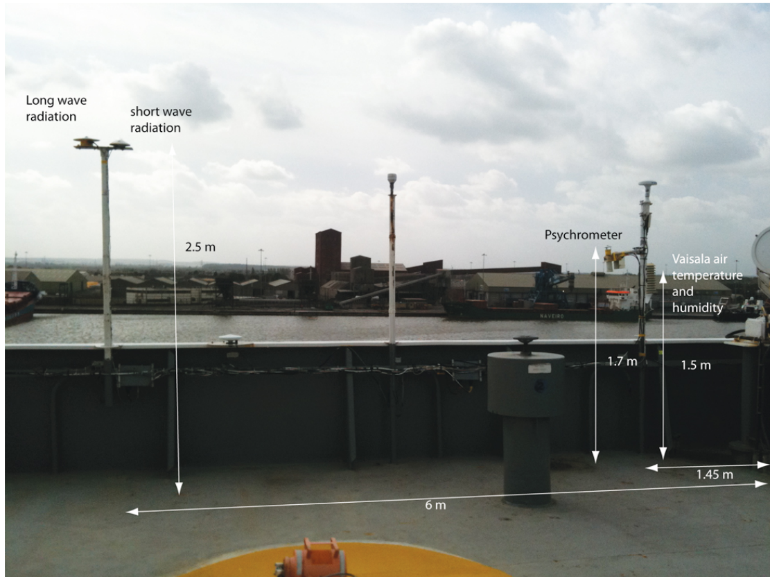
Figure 4 Photo of the mean meteorological sensors on the bridge top. Photo taken in Immingham, UK on the 3rd October 2011.
