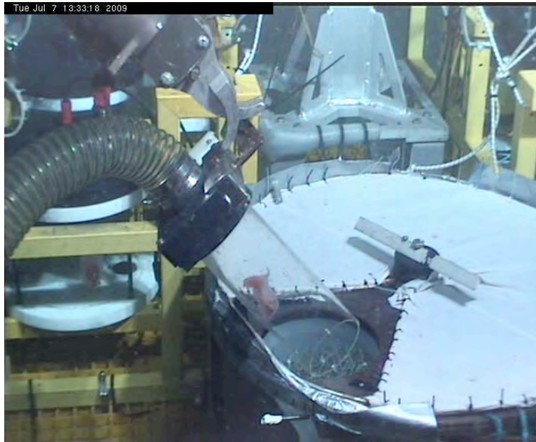
Figure 3. ISIS suction sampler putting a specimen of Peniagone sp. in the experimental apparatus.
