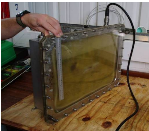
Figure 2 - A pressure balanced battery.
