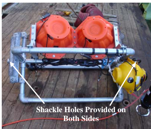
11 a – Assembled and Enhanced Scaffolding Frame
