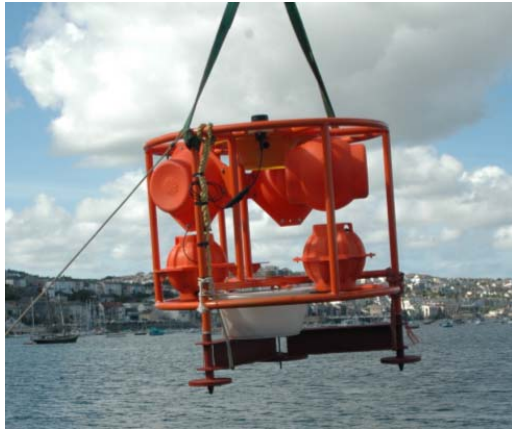
a – MYRTLE Plus Ballast Weight Lowered from the Aft Deck of Discovery
