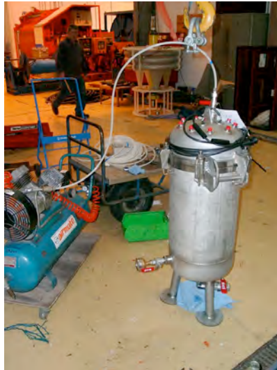
The SNOMS tank under leak testing at NOC
