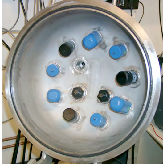
The Aanderaa sensors for temperature, conductivity and dissolved oxygen newly fitted into the lid of the SNOMS tank
