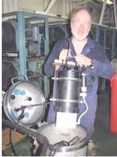
The ProOceanus ProCO 2 unit being lowered into the SNOMS tank prior to the test cruise on the Pride of Bilbao.
