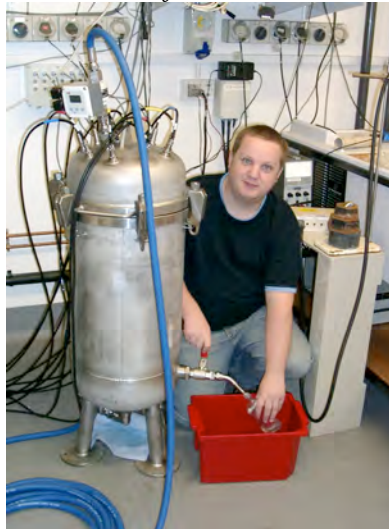
Dave Childs collects a sample to of the seawater being pumped through the tank so he can measure its salinity to compare with the output from the Aanderaa sensors
