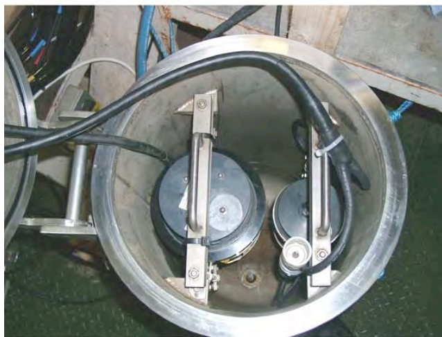
Interior of OceanBox tank after cleaning. Tank contains the ProOceanus ProCO 2 and GTD units. The Seabird 38 thermometer(used for comparison with the Aanderaa 4050 thermometers in the lid of the tank) can be seen at "5 o'clock".
