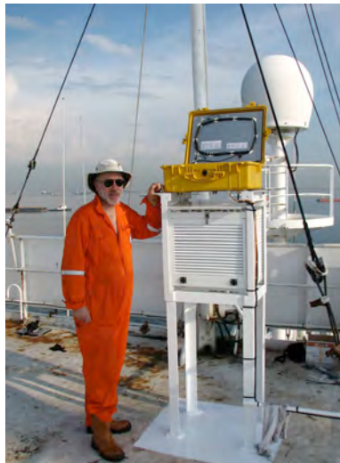
Stevenson Screen and Iridium GPS box on the frame on the Monkey Island
