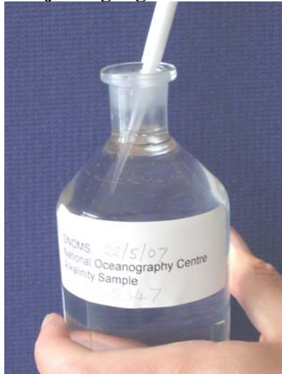
Close up of position of tip when injecting \text{HgCl}_2 solution
