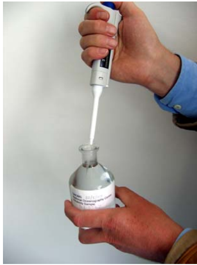
Close up of position of tip when injecting \text{HgCl}_2 solution
