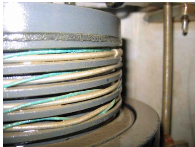
11 Place camera in tank to photograph ProCO2 sensor coil head. (One from Pride of Bilbao - A much lower level of fouling is expected on the Pacific Celebes. If you see anything like this please let us know)
