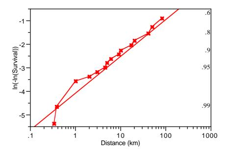
**Figure 3** Probability plot for the 'All missions' data set with that estimated from a Weibull distribution with  $\alpha = 403.9$  and  $\beta = 0.678$ . The right hand scale shows the probability of survival.
