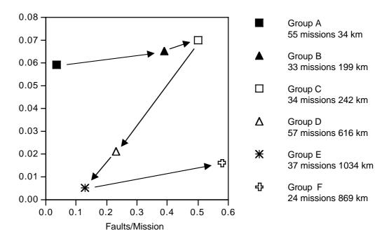
**Figure 2** Time history of the faults per km and the faults per mission for the six groups of missions. The arrowheads show the progression in time from Group A to Group F.
