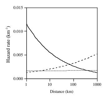
**Figure 4** Hazard rate as a function of distance travelled from the Weibull model for the 'All missions' group, all faults (solid line), for the seven high impact underway faults that would have led to loss in a covered ocean (dashed line) and for the five non-terrain following underway faults (dotted line).
