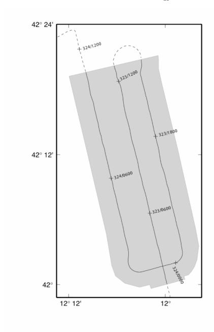
Figure 4. Track chart and TOBI sidescan sonar coverage (shaded) for the *Prestige* study area. Solid track lines are those along which sidescan data was acquired, dotted lines are passage tracks.
