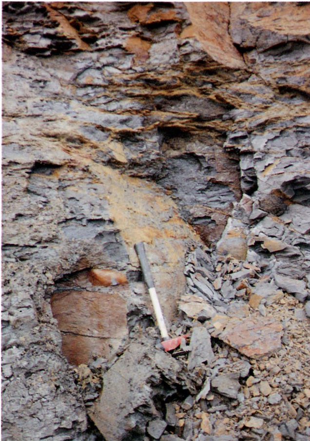
Plate 2 Selbourne Brickworks. Weathered, desiccated highly fissured Gault clay with water flowing through the oxidised fissures.
