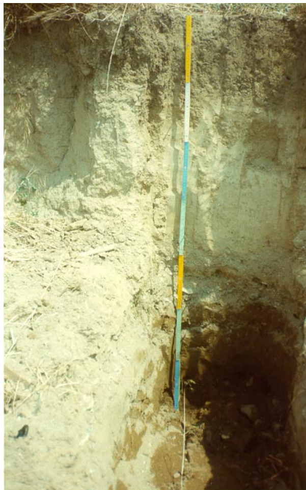
Fig. 12. Floodplain sediment sequence with soil development in Greece. Meter: coloured sections 20 cm. Fine-grained clay and silt down to a depth of 75 cm (low energy floodplain sediment - good for sampling; soil has developed down to a depth of 25-29 cm). Coarse-grained sandy and bebbly unit between 75-100 cm (high energy environment). Sandy-clay unit between 100-134 cm (low-energy environment). Gravel bed below a depth of 134 cm. Photo: A. Demetriades, IGME.
