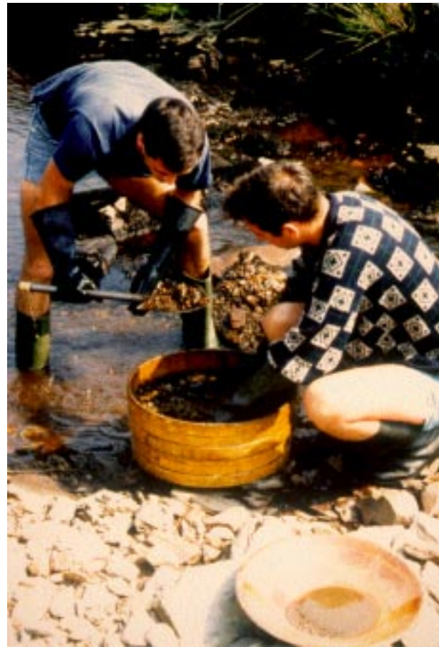
Fig. 7. Wet sieving of a stream sediment sample (Photo: Fiona Fordyce, BGS)
