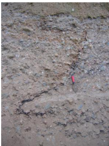
Plate 18 Riereach Burn Site 4, location CA4135. Iron and manganese staining along Redox front developed in deeply decomposed gravel. Trowel 17 cm long. [GR 284605, 844123]
