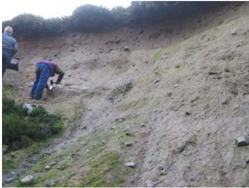
Plate 21 Drynachan Burn Site 1 (West Section), equivalent to Section NH83NE E1. Sampling in silty grey brown/light olive brown lodgement till. [GR 285987 839975]
