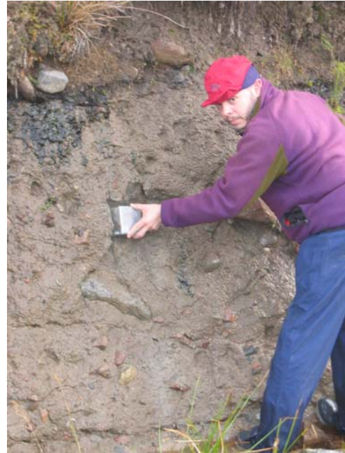
Plate 10 Riereach Burn Site 1, Section NH84SW E17. Micromorphology sampling of grey-brown basal granite/psammite-rich suglacial till. Kubiens sample tin 10cm x 10 cm. (Sample 3).
