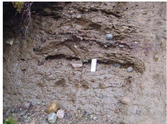
Plate 25 Drynachan Burn Site 2 (East Section), equivalent to Section NH83NE E1. Upper strongly laminated, very stiff slightly gravely, silty till. Scale 10cm long. [GR 286030, 839900]
