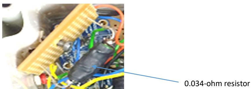
Figure 45. Inner wiring of the monitoring unit showing the 0.034-ohm resistor.
