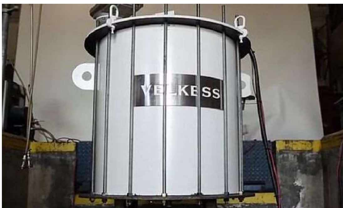
Figure 24. Velkess flywheel energy storage [10].
