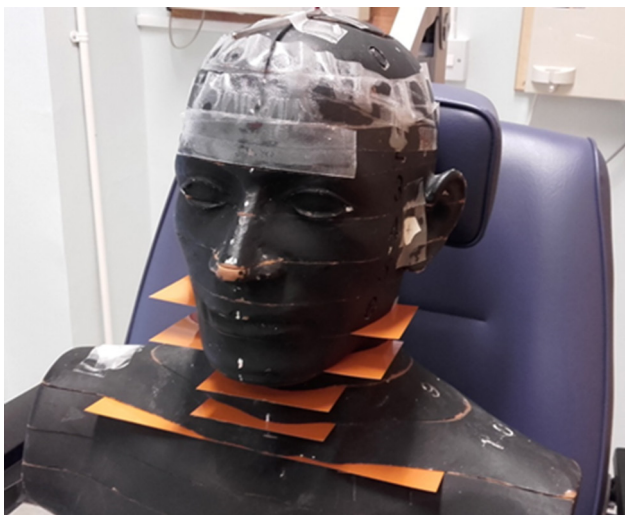
Figure 1 The XRQA Gafchromic film positioned within the Rando phantom.
