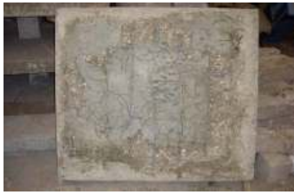
(a) Slab S1; ordinary concrete without steel fibres
