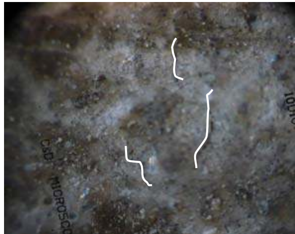
Figure 6 Shrinkage cracking on cigarette filter concrete
