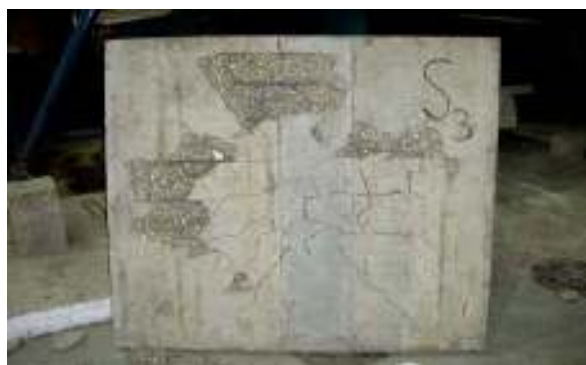
(c) Slab S3; HSCC without steel fibres
