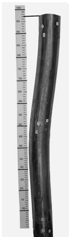
Figure 3 Concrete-filled steel tube column of height 100 cm and diameter 102 mm with wall thickness 3 mm after the third impact by 480 kg weight falling from 210 cm height
