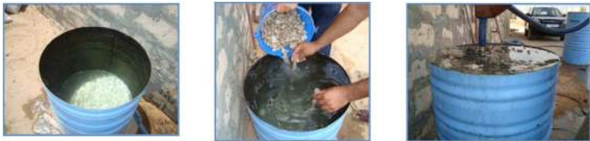
Figure 5 Underwater concreting by using two stage concrete
