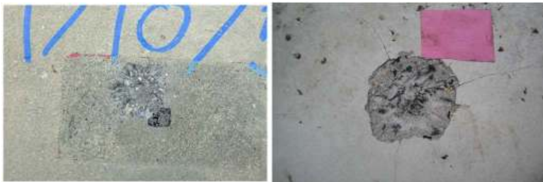
Figure 5 Failure Patterns of SFRC plate (left) and CRC+SFRC plate (right)
