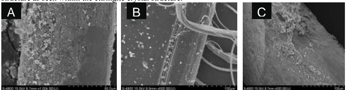
Figure 13 SEM images of fibres pulled from the OPC matrix: (A) PVA (1000x magnification); (B) PP (500x mag); (C) Steel (500x mag)
