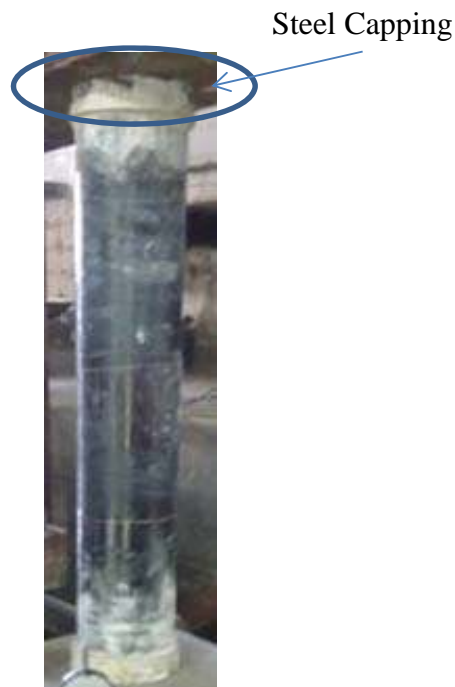
Figure 2 Confined column with steel capping before loading
