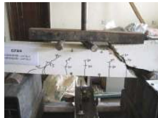
Figure 13 mode of failure GFB9
