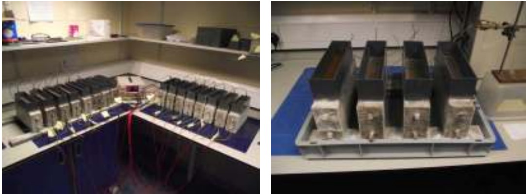
Figure 1 experimental setup for determination of corrosion rates
