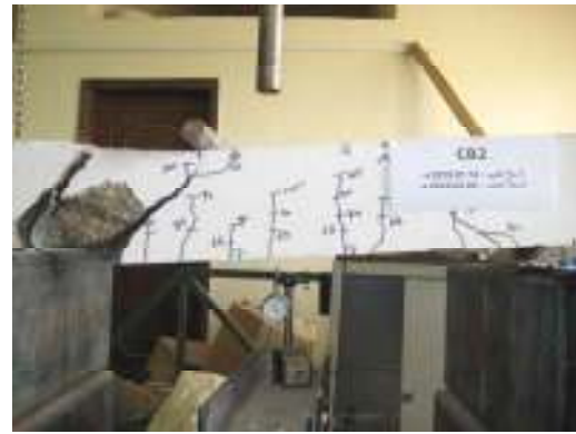
Figure 15 mode of failure CB2
