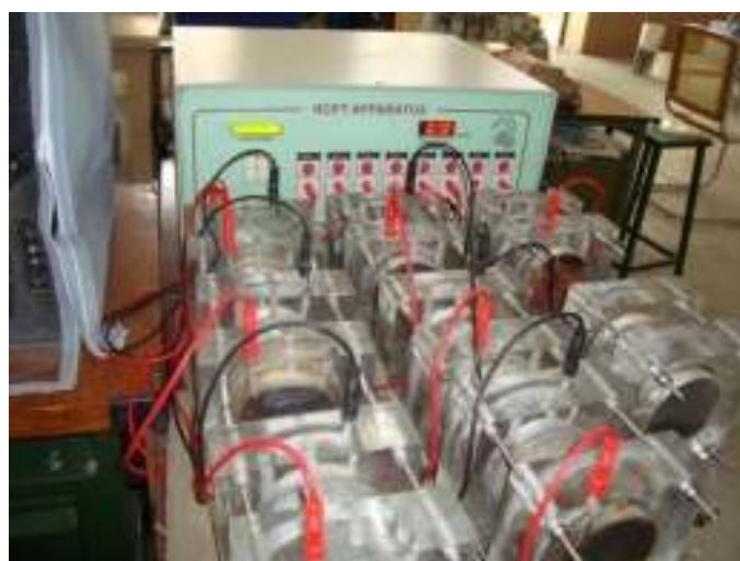
Figure 1 Multi-cell RCPT Apparatus with specimens
