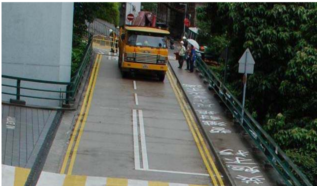
Figure 6 Lorry for verification load tests
