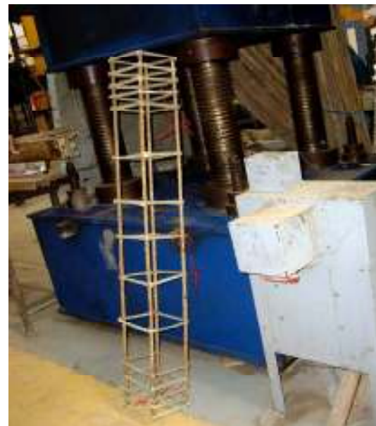
General view of GFRP bars and stirrups
