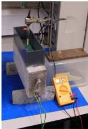
Figure 2 half-cell measurements for corrosion initiation
