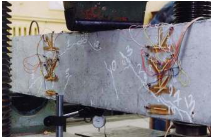
Figure 3 A three-point bending of concrete beam specimen
