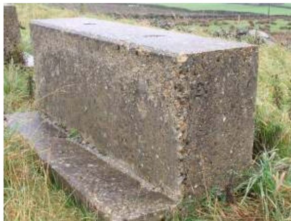
Figure 2 Non air-entrained 30 MPa Portland cement concrete exposed for 12 years and around 1100 freeze thaw cycles as measured by air temperature
