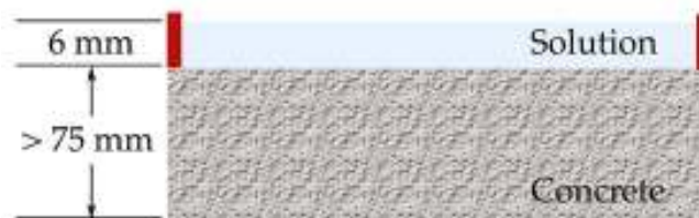
Figure 2 Laboratory scaling specimen with Styrofoam dike applied
