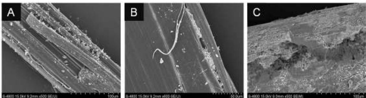
Figure 21 SEM images of fibres pulled from the CAER CSAB matrix: (A) PVA (500x magnification); (B) PP (600x mag); (C) Steel (500x mag)
