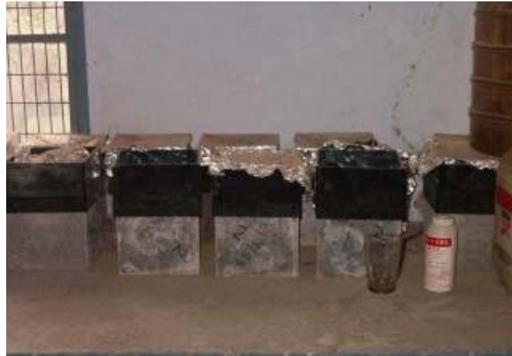
Figure 1 Dykes prepared at the top of the specimens for ponding chloride solution
