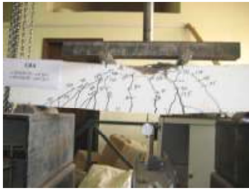
Figure 16 mode of failure CB4
