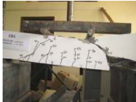
Figure 9 mode of failure CB1
