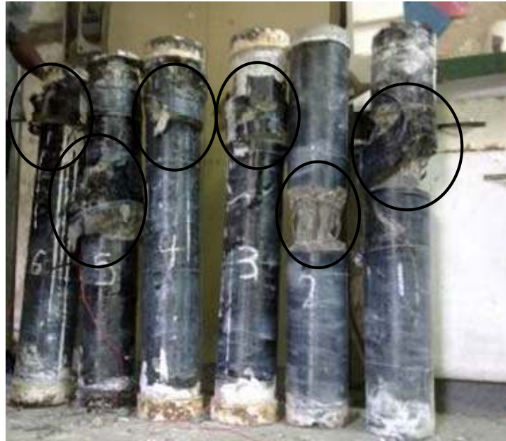
Figure 6 Failure modes for all columns
