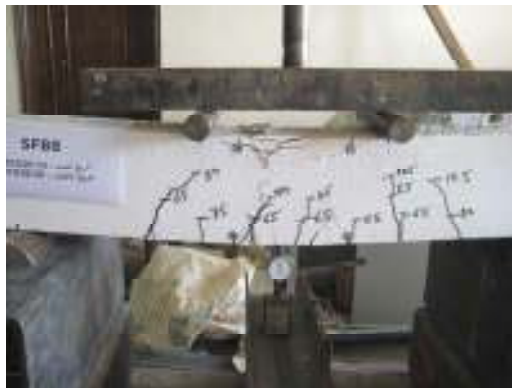
Figure 18 mode of failure SFB8
