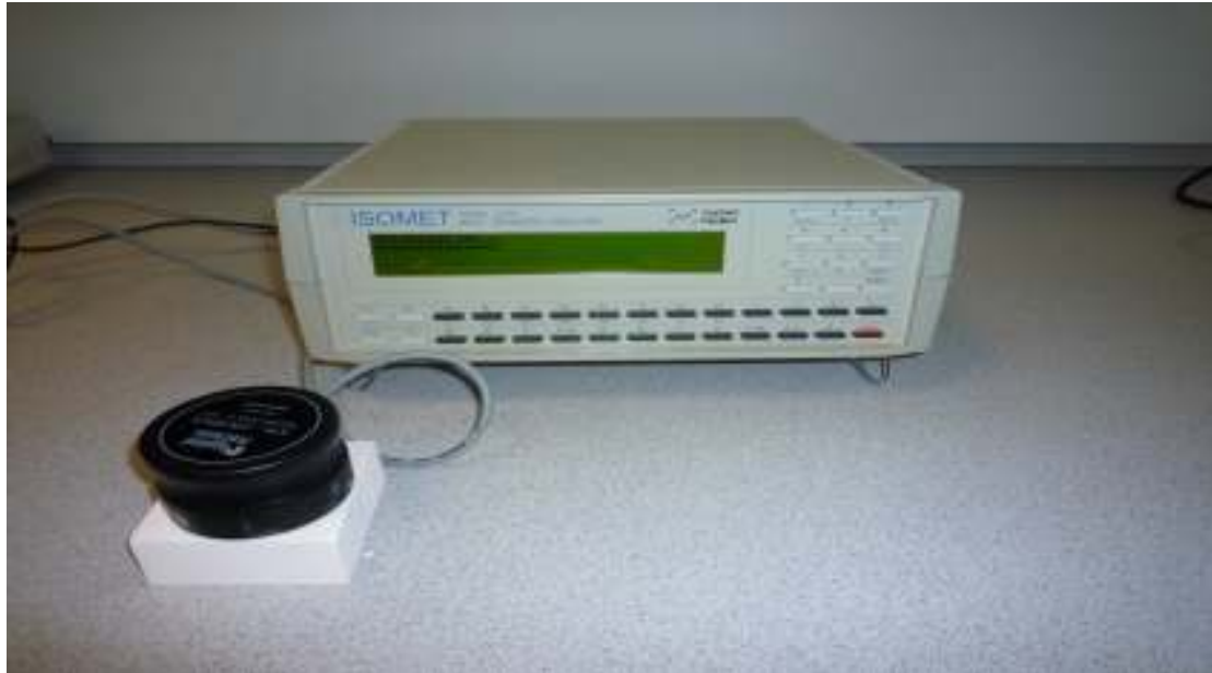
Figure 2 Apparatus for measurement of thermal properties - ISOMET 2114
