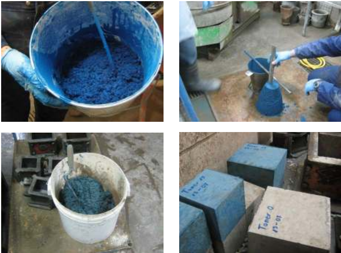
Figure 3 Mixing concrete coloured with cyan toner
