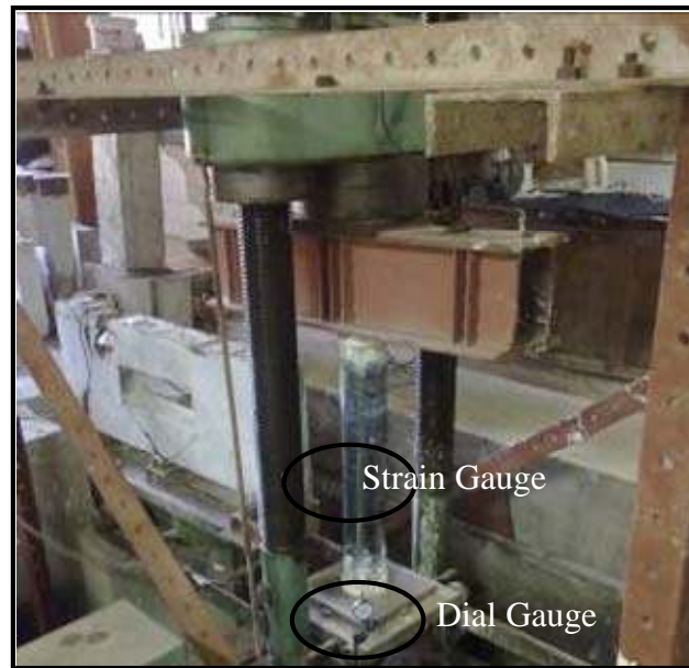
Figure 3 Test Setup and column instrumentation
