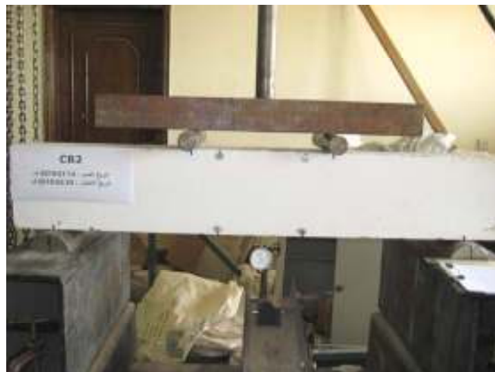
Figure 3 Model of the concrete beams load test
