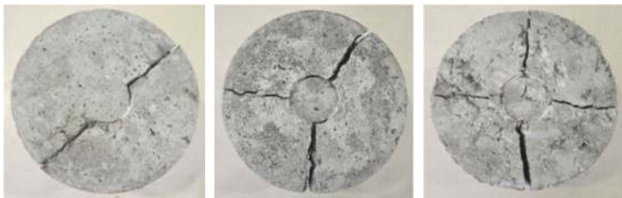
Figure 3 Final specimens state with typical cracks patterns
