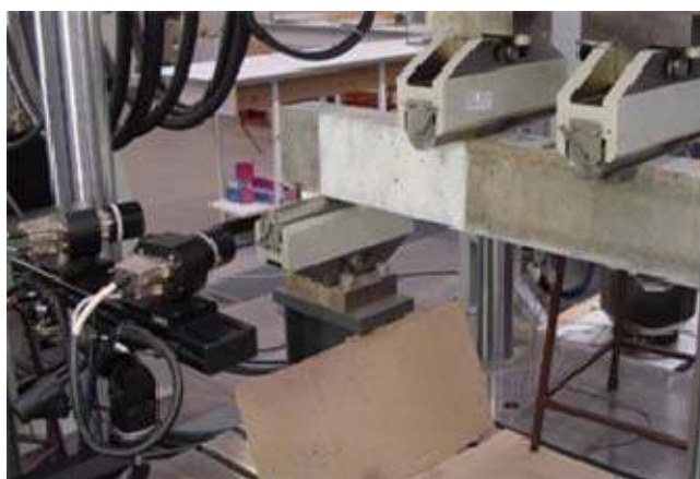
Figure 4 Experimental set-up of the test specimens and the video camera
