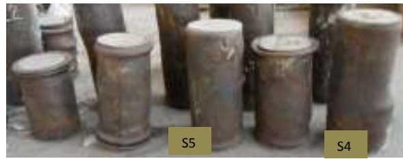
Figure 4 Buckling of the tube wall
