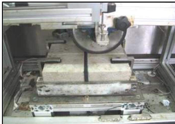
Figure 3 Configuration of wheel tracker machine
