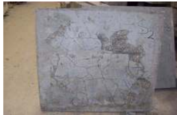
(b) Slab S2; SCC without steel fibres
