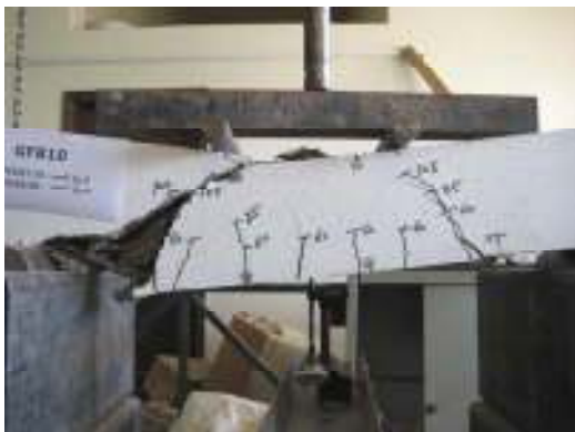
Figure 19 mode of failure GFB10
