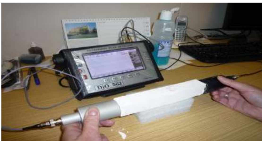
Figure 3 Apparatus for measurement of modulus of elasticity - DIO 526
