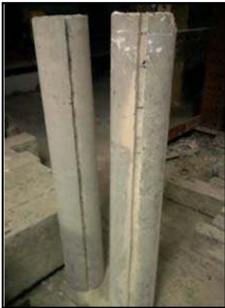
Figure 5 Failure and first crack loads and embedding the external reinforcement into the column concrete cover
