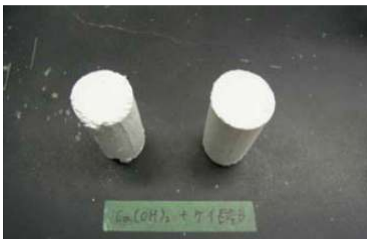
Figure 1 Hardened specimen of calcium hydroxide
