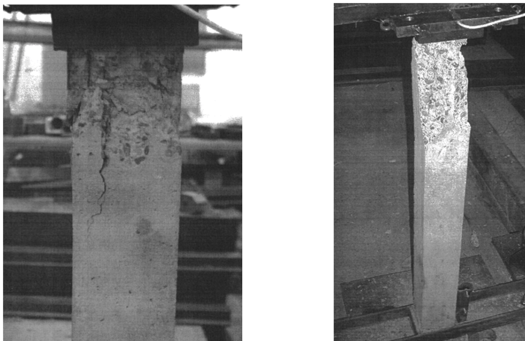
Figure 1 Patterns of the model fracture after second impact by 225 kg weight falling from 35 cm height: left — co-axial impact; right — angled impact
