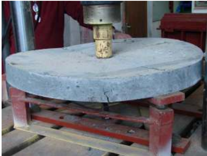
Figure 2 Round disc test setup
