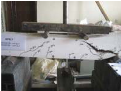
Figure 12 mode of failure SFB7
