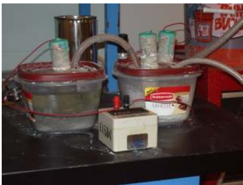
Figure 2 Rapid macrocell test setup
