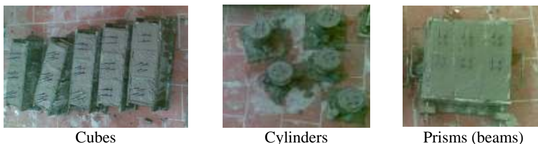
Figure 2 The specimens after casting and installing probes
