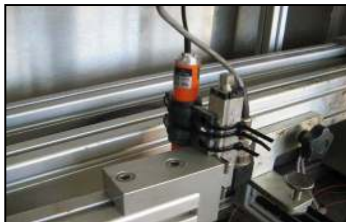
Figure 7 Additional TML LVDT for tests
