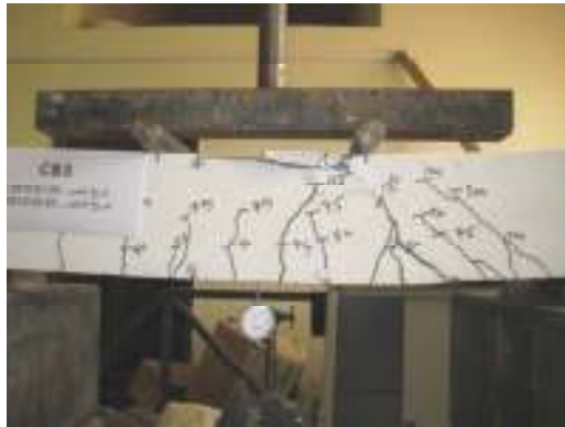
Figure 10 mode of failure CB3
