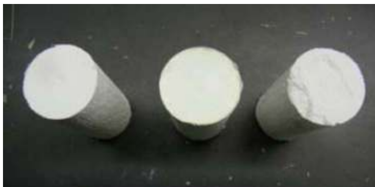
Figure 2 Hardened specimen of calcium carbonate
