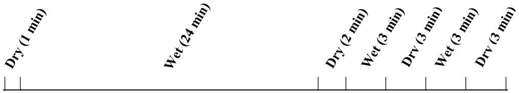
Figure 121: Timeline of the movement of the sweat capsule between the dry and wet docking chambers.
