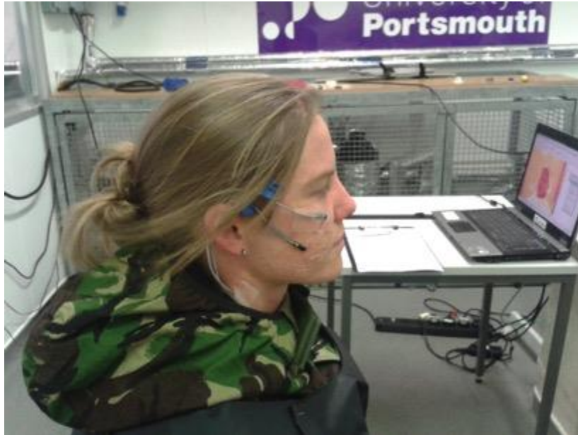
Figure 72: The participant resting in a hot and dry chamber wearing a full military chemical protective ensemble (without the hood or respirator) with two skin surface thermistors attached to the right cheek with either a Tegaderm TM (lower thermistor) or Transpore TM (upper thermistor) tape.
