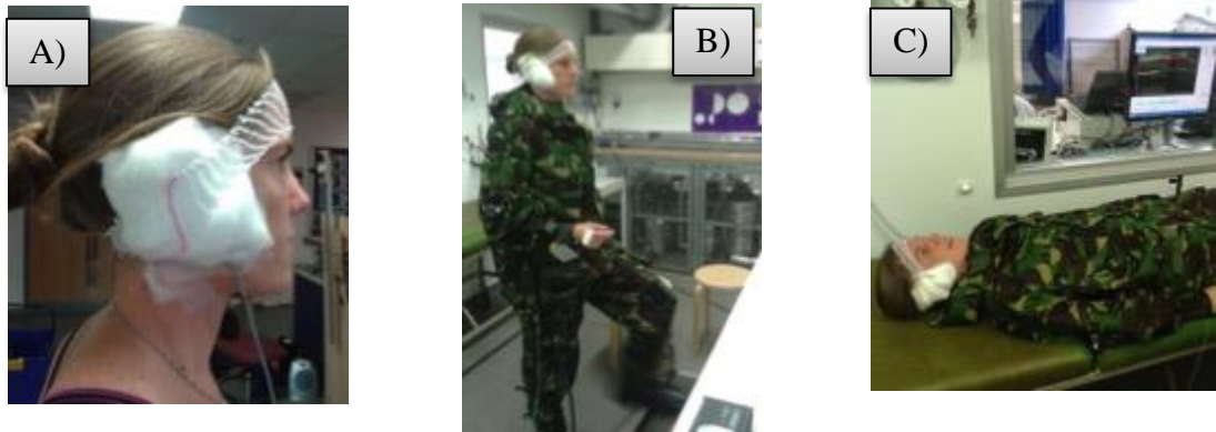
Figure 135: Measuring core temperature using an aural thermistor. A) A participant instrumented with an aural thermistor, B) a participant stepping, C) a participant lying down supine.
