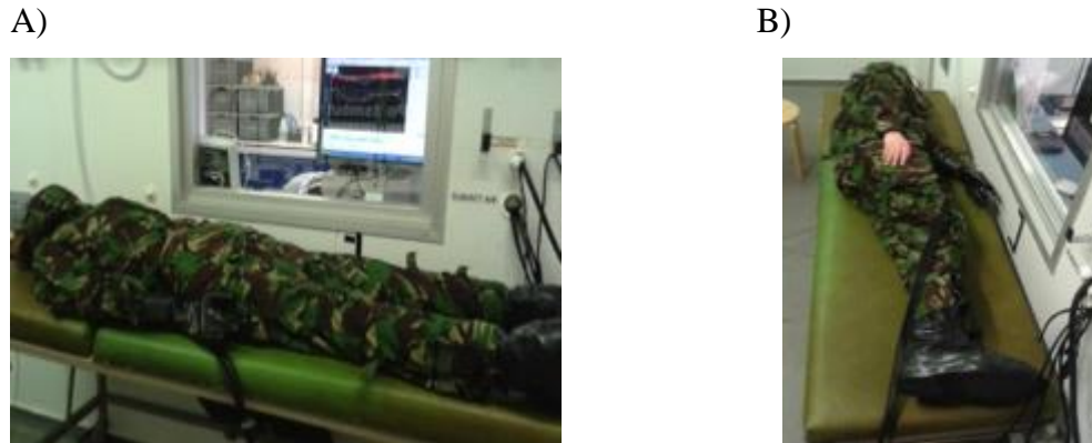
Figure 114: A participant adopting the prone (A) and lying down on the left side (B) postures whilst wearing chemical protective clothing without the respirator and hood in 40.0 °C and 40 % rh air.
