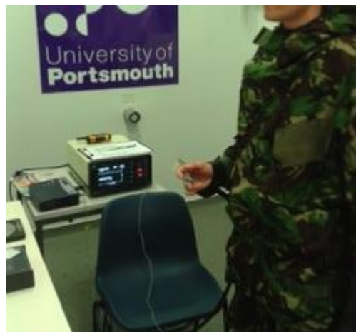
Figure 115: A participant instrumented with a beat-to-beat blood pressure monitoring device on the right middle finger to detect hypotension during standing whilst wearing chemical protective clothing without the respirator and hood in an environmental chamber set to 40.0 °C and 40 % rh air.
