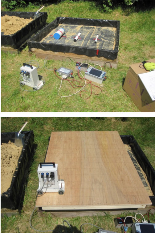
Fig. 2. Experimental setup and GPR equipment used in the experiment
