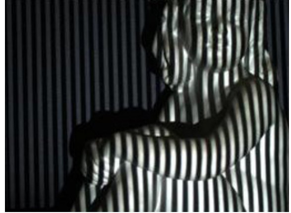
Figure 3 The principle of Lightcoding
