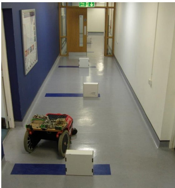
Fig. 1 The tele-operated mobile robot being remotely driven along a corridor
