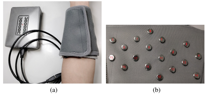
Fig. 1. This picture shows the device used in this experiment. (a) A muscle electrical apparatus comprising 16 channels, which can be used to gather single channel data or be matched with electrode sleeve for multi-channel data acquisition. (b) Electrode sleeve, which contains 18 electrodes altogether (The number 9 and 10 are two reference electrodes, and the remaining are 16 signal channels). It can be divided into two connected rings: 1-8 for one, and 11-18 for the other. This electrodes configuration was named Zig Configuration.
