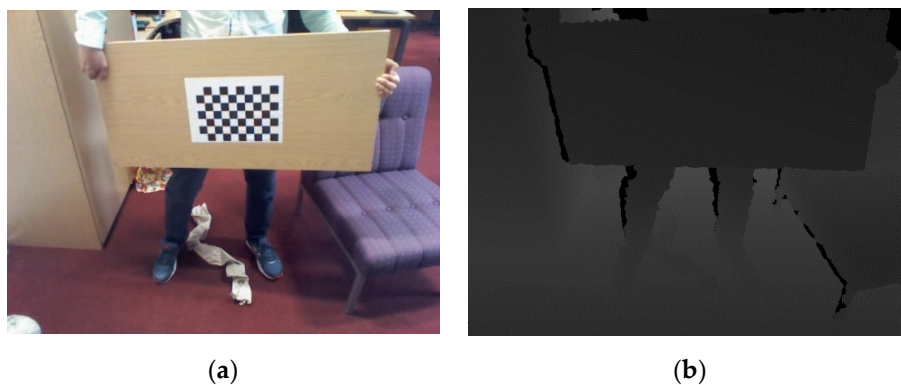
Figure 9. One of the test data sets. (a) the checkerboard image under Kinect view; (b) the corresponding depth image.
