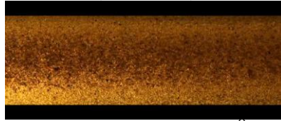
Figure 6: Sand transport condition for oil (340 cP at 16 o C) and for 200 lb/1000 bbl, V_{oil}=0.25\text{ m/s} (Bottom view)
