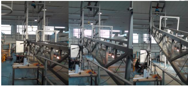
Figure 3: 4-inch test facility tilted at 5, 10 and 20 degrees
