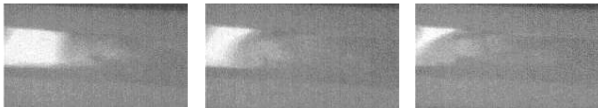
Figure 7. Real Time X-ray of highly entraining return wave propagating along the channel
