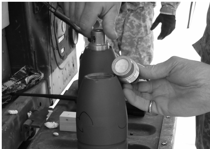
Figure 2. Installing fuze simulators in 81-mm mortar rounds. Note C4 explosive in base of simulator and hole for blasting cap on top of the simulator.
