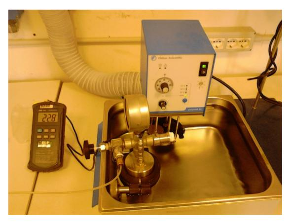
Figure 3-2 The equipment used for the batch carbonation tests.
