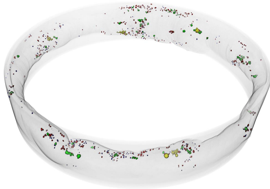
Figure 30: Weak fusion area
