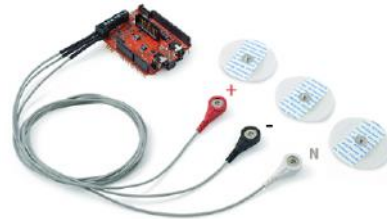
Figure 3-2: E-health Arduino Shield with ECG sensor leads connected on it.
