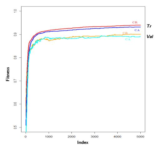
Fig. 7.9: Comparison of class predictive accuracy between the CA and CR methods for training (Tr) and validation (Val) data. The CR method provides higher predictive accuracy than the CA method, with a difference of around 1%.
