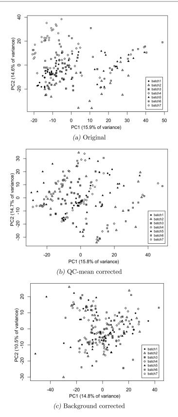
Fig. 4.1: (a) The scores plot for the first two principal components of the scaled L+ dataset showing batch differences as a major source of variation. (b) The scores plot after batch correction using the mean QC value, in which batch differences are made worse. (c) The scores plot after batch correction using the background correction method, in which batch differences are no longer apparent.
