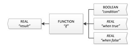
Fig. 7.4: Strong-typed If statement tree showing input types expected (bottom) and output type produced (top).
