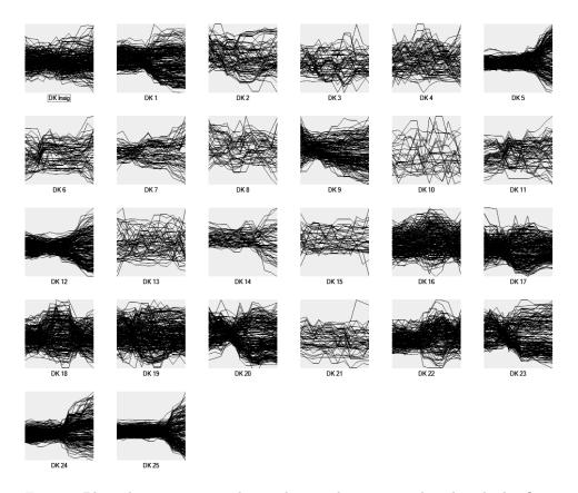
Fig. 5.6: Plots showing vectors clustered using k-means combined with the Qian distance metric. The x-axes of the plots denote time, whilst the y-axes denote intensity. Whilst several of the clusters display noticeable trends over time, a number of clusters display noisy profiles due to the presence of samples grouped together by spurious data-points.
