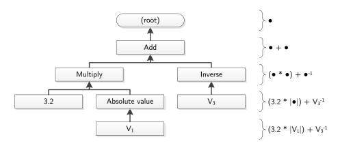
Fig. 7.1: Example of a genetic programming tree, representing the equation  $(3.2 * |V_1|) + V_3^{-1}$ .
