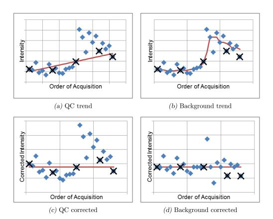
Fig. 4.2: Plots showing how two methods of correction affect a metabolite  $(\mathcal{L} + \#3280)$  and batch showing strong within-batch drift. Plots (a) and (b) show the values prior to correction, with the trend used for the two different correction methods shown by the bold line. Figures (c) and (d) show the values post-correction, with the bold trend-line at 1.0. The linear correction (c) shows a notable pattern in the results when compared with the moving median correction in (d).
