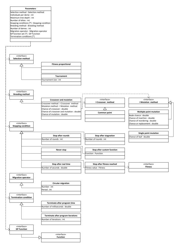
Fig. 7.5: UML diagram showing the parameters available for modification in a typical ST-GP simulation, along with the dependencies of parameters upon each other.
