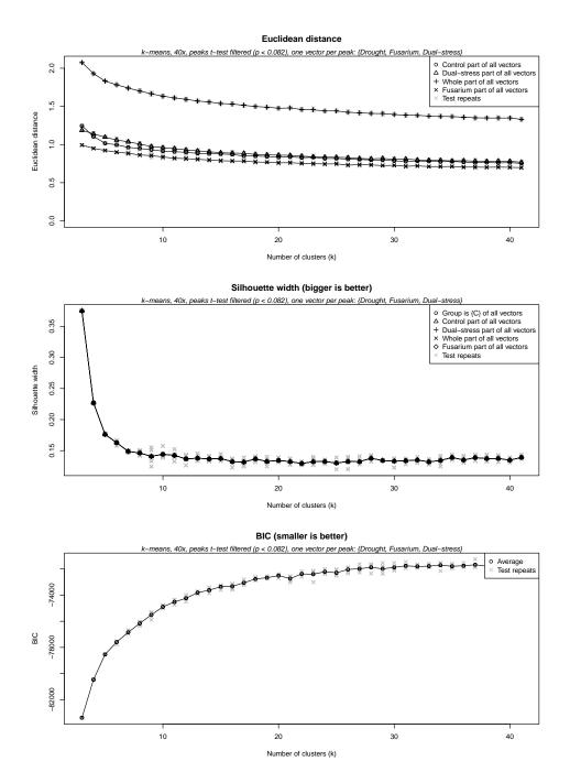
Fig. 6.6: Results of various runs of the k-means clustering algorithm, displayed in terms of two measures of performance: Silhouette width and BIC. The average euclidean distance from the cluster centres is also shown for comparison. These results show decreasing performance with increasing k.
