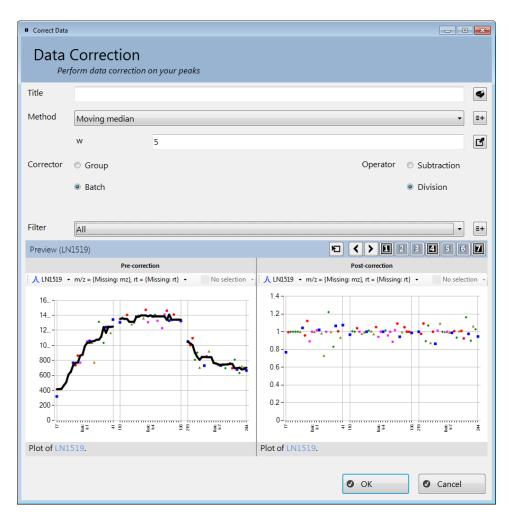
Fig. 6.4: Image showing the in-software preview displayed for a moving median batch correction (window width = 5) of a particular peak. The post-data correction can be seen to be free of the changes in intensity (Y) with acquisition order and batch (X) that are encountered if a linear correction model is used.
