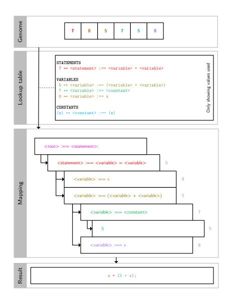
*Fig.* 7.3: Depiction showing the translation of an arbitrary byte-based genome through a set of BNF syntax rules into a compilable segment of code.
