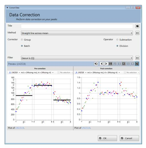
Fig. 6.3: Image showing the in-software preview displayed for a mean-of-the-QCs batch correction. Variations in intensity (Y) between batches and along the acquisition order axis (X) can be seen post-correction.
