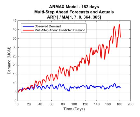
Figure 6.4: Multi-Step Ahead Forecast for model AR(1)/MA(1,7,8,364,365)
