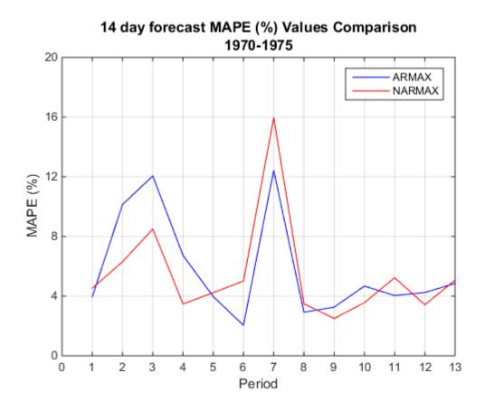
Figure 6.17: 14-day ahead Forecast - MAPE (%) Values Comparison ARMAX vs NARMAX
