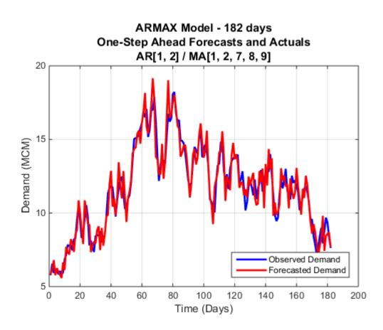
Figure 6.12: One-Step Ahead Forecast for model AR(1,2)/MA(1,2,7,8,9)
