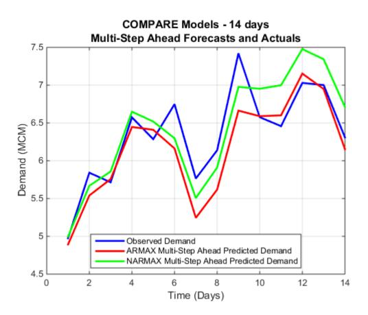
Figure 6.18: Period 1 - 14 Day Multi-Step Ahead Forecast - Comparison ARMAX vs NARMAX
