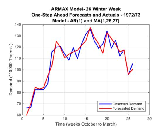
Figure 5.15: One-Step Ahead Forecast for model AR(1)/MA(1,26,27)
