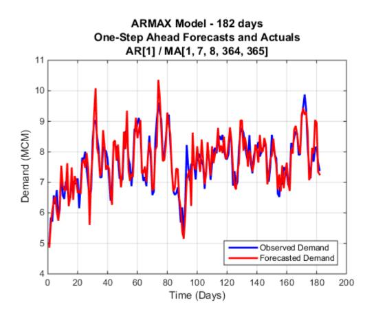
Figure 6.3: One-Step Ahead Forecast for model AR(1)/MA(1,7,8,364,365)
