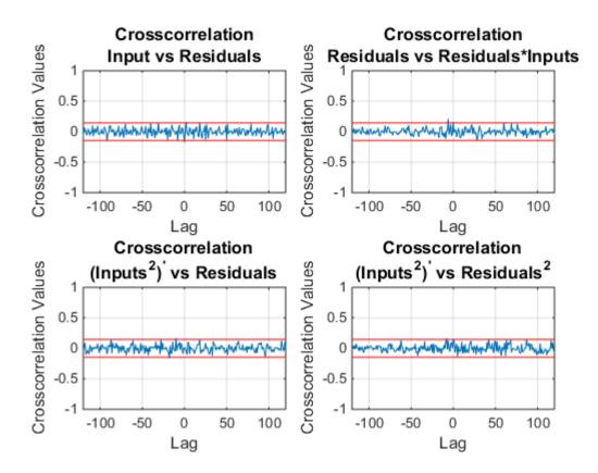
Figure 5.18: Linear and Non-Linear Validity Tests
