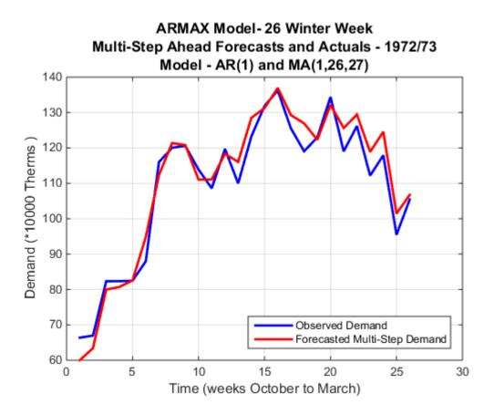
Figure 5.16: Multi-Step Ahead Forecast for model AR(1)/MA(1,26,27)
