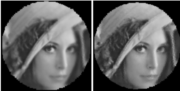
Figure 3: Backprojected retinal images. Left: a well-parametrized retina. Right: a badly parametrized retina. Note the jaggy edges at the peripheries of the right image.
