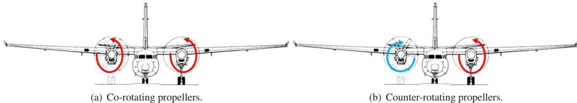
Figure 2: Propeller rotational direction definition.
