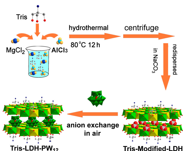
Figure 4. Schematic representation of the host layer modification method to prepare POM-LDH composite (Tris-LDH-PW 12 ). Adapted from Ref. [41], Copyright 2014, Royal Society of Chemistry.
