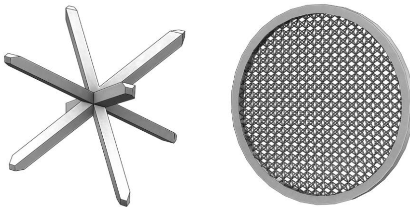
Figure 1: Lattice unit cell and the 1-layer disc filter.
