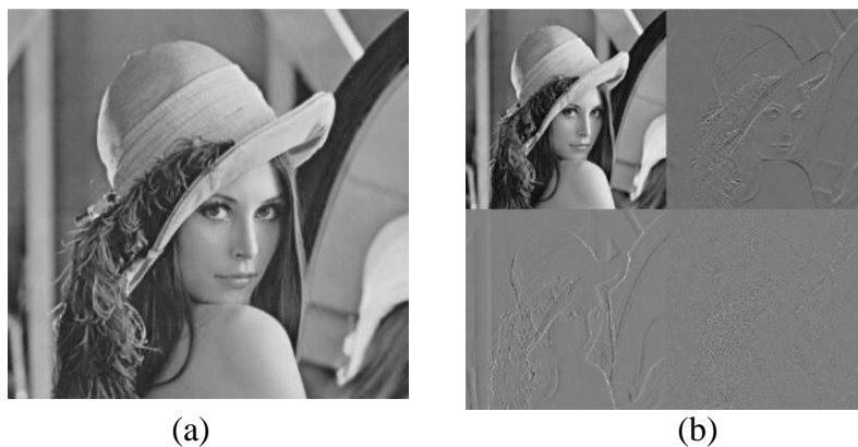
Figure 2-3 One-step 2-D wavelet decomposition: (a) original image, (b) Decomposed image.
