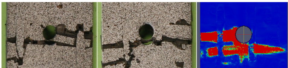
Fig. 24. A comparison of the matrix cracking pattern observed in two experimental samples against the model predictions (surface of the experiments is speckle painted for digital image correlation (DIC) measurements).
