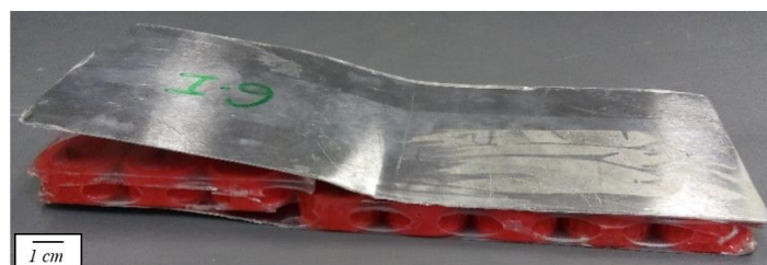
Figure 10. A bottle caps sandwich sample with core shear failure between the adjacent caps.
