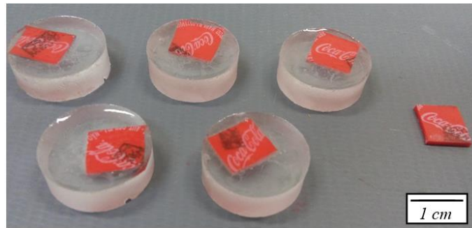
Figure 6. Bottle caps samples used in the microhardness test
