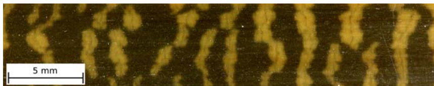
Figure 2. Striped pattern indicating carbon ply fragmentation triggered by overload in a glass/carbon hybrid specimen [5]
