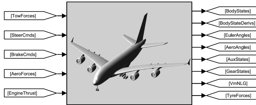
Fig. 1 Top-level SimMechanics model of an A380. Reproduced from [4].
