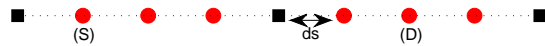
Fig. 1. Example illustration of user mobility with N=3 and N_d=4 . Lattice points are the squares and the densification points are the circles. The user speed is v = 1 thus, dt = \frac{1}{4} . Source and destination points are indicated by (S) and (D). Travel starts at t = 0 . The user reaches the destination at t = 5dt . The user location at t = 4dt is used to compute the correlation at \tau = 1 .
