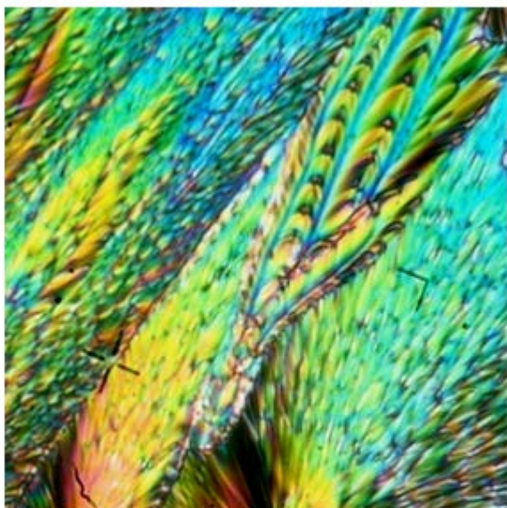
Figure 2. (colour online) The optical texture for the N_{TB} phase of 10.3.O1 at 30°C supercooled from the isotropic phase. The sample was contained between thin and untreated glass slides.
