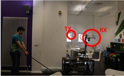
Figure 3: Measurement location, showing transmitter, receiver and corner under investigation.
